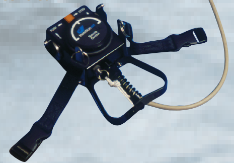
Hand-held remote for "walk-about" manoeuvring control
